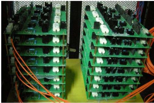
Fig. 7. Assembled IGBT stacks which are composed of 64 series-connected IGBTs.
