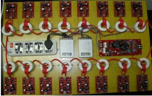
Fig. 4. 50-kV isolation auxiliary power supply for IGBT stacks.
